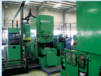
Tooth profile processing
